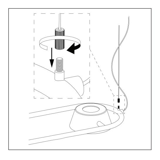
Take off the internal bracket from the canopy and the hanger bases from two steel wires. Fix the bracket and hanger base on the ceiling. The center distance between two hangers is 1336 mm / 52.6 inches.
