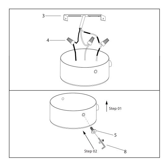
Screw the wire in the base of the frame.
